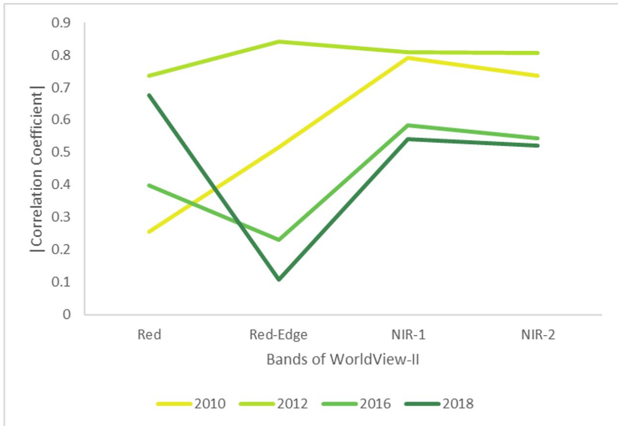
Fig. 4. The absolute values of correlation coefficients of canopy density assessed from GMSV and the pixel values of the Worldview-II satellite bands across all four years examined.
